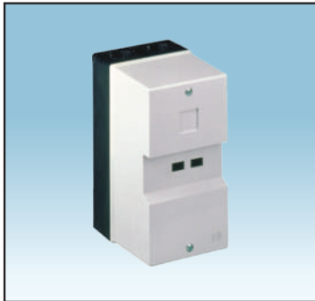
Insulated enclosure IP 41 with integrated PE(N) terminal top and bottom each 2 metric knock-outs
